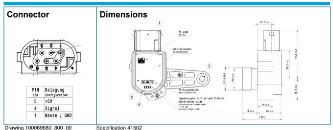
IP 6K9K (with fitted Output - voltage (0.5 ... 4.5) V Supply Sealing grade female connector) range Temperature -40 °C to 100 °C ± 45° **Output signal** Angle range 1 signal (analog) range AMP No. 114-18063-21 (coding A) Current gold plated, Independent linearity ≤ 1 % Max 5.5 mA Connector consumption Female connector on request Signal characteristic curve
